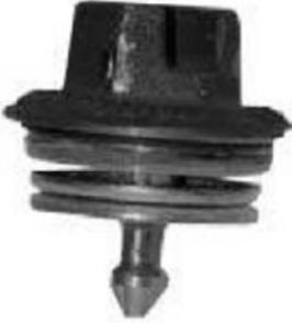
1. Remove the cap of the steam trap (*turn it counter-clockwise*).
