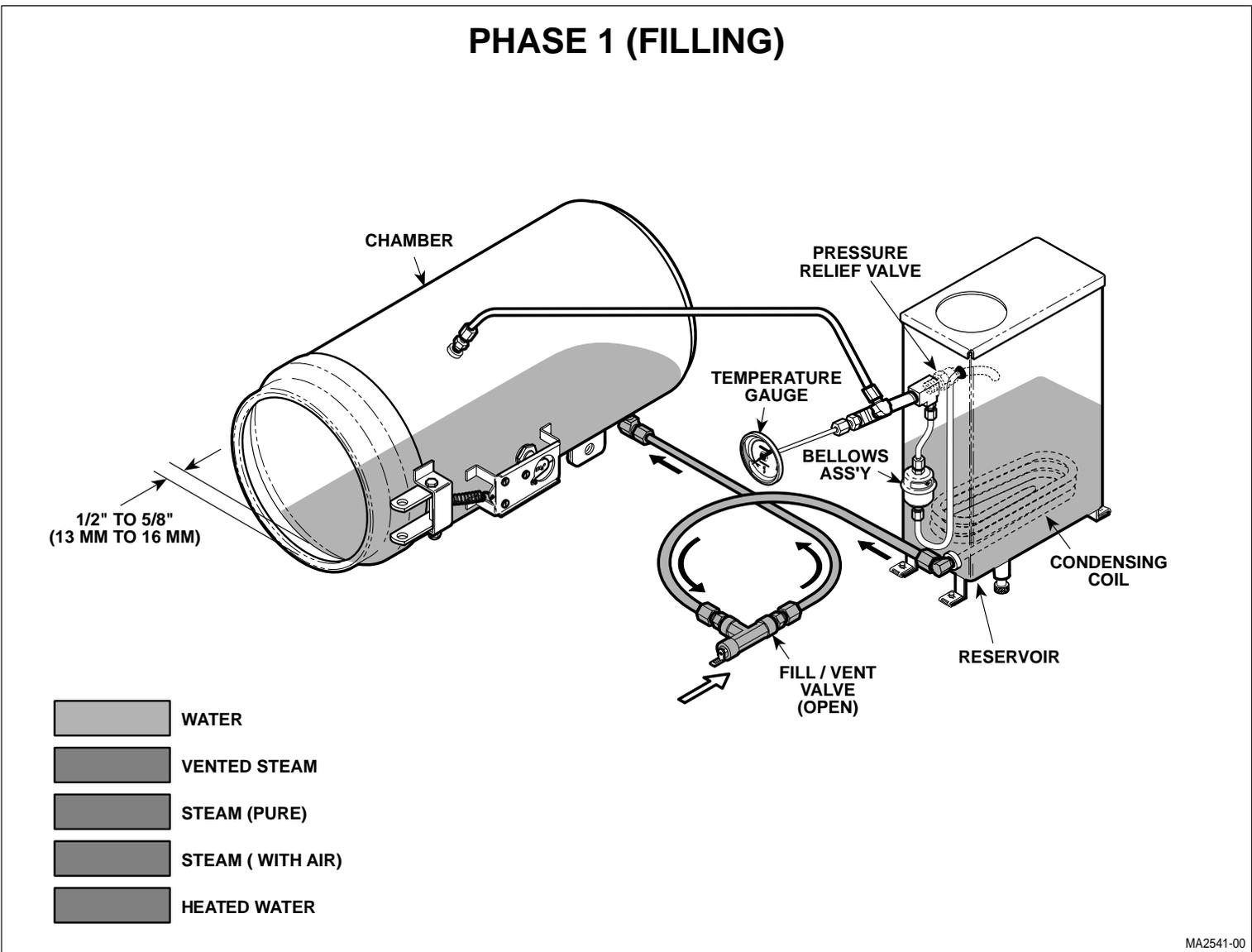
Figure 5-3 (Sheet 1 of 4). Flow Diagram
