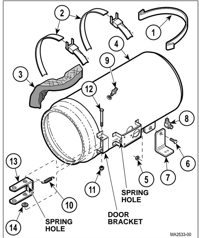
**Figure 4-26. Chamber Assembly
