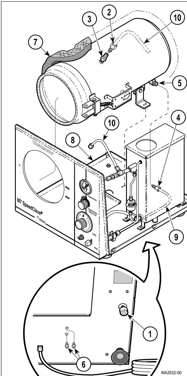
**Figure 4-25. Chamber Assembly
