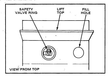
WARNING: When ring is pulled on safety valve with unit under pressure, steam is discharged from the chamber at a high temperature. Keep clear of steam discharge path to avoid burns. Use of a hot pad or instrument to pull ring is suggested.
